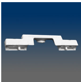
8288 Keeper, sash, surface mount, #6 screw, 2.25" C/L, with pegs at the bottom, open back, material: zinc alloy
