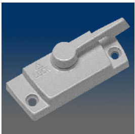
3222 Sash lock, surface mount, 2.062" C/L, .688" setback, #6 screw
