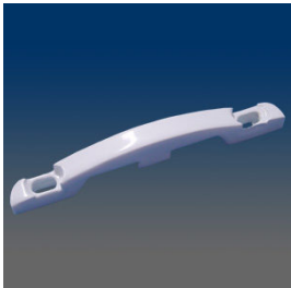
9356A Keeper, sash, surface mount, for non-hooded 600 series hooded lock, #6 screw, 2.062" C/L, closed back, material: zinc alloy
