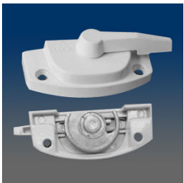
3225DB Sash lock, surface mount, 1.875" C/L, .688" setback, #6 screw, snap-back lock, unique spring design eliminates exposing the cam in the partially open position
