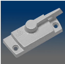
3222 Sash lock, surface mount, 2.062" C/L, .688" setback, #6 screw
