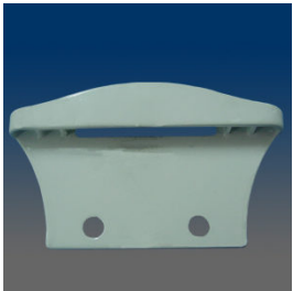
9354 Keeper, sash, face mount, for 600 series non-hooded lock, #8 screw, 1" C/L, material: zinc alloy
