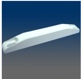
9382 Keeper, sash, surface mount, #6 screw, 2.25" C/L, closed back, material: zinc alloy, match with 9280 lock
